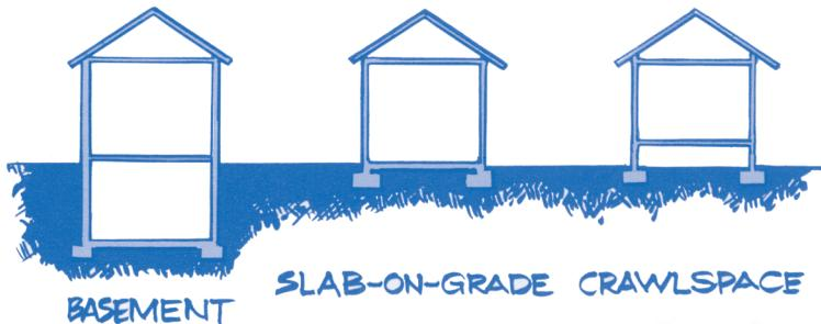
Radon reduction systems can be grouped by home foundation design. Find your type of foundation design above and read about which radon reduction systems may be best for your home.
